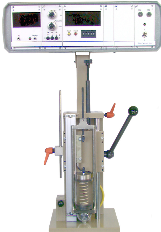
Picture: Load tester WG 3/3 available with specified load ranges:
